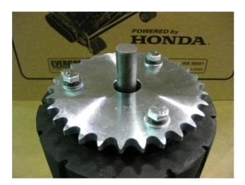
Make sure the roller spins freely. If prior to installation of the "30 Tooth" sprocket the roller spun freely, but now does not, add a washer under each of the spacers.
