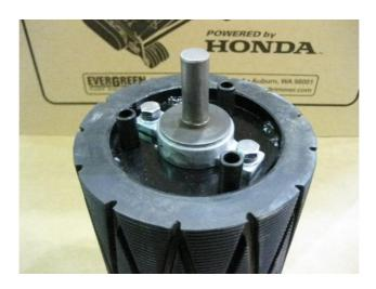
Install a "30 Tooth" sprocket using the bolts, lock washers and washers. Try to center the sprocket as much as possible.
