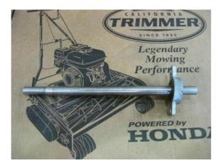
One end plate on the roller is set deeper inside the roller than the other.
