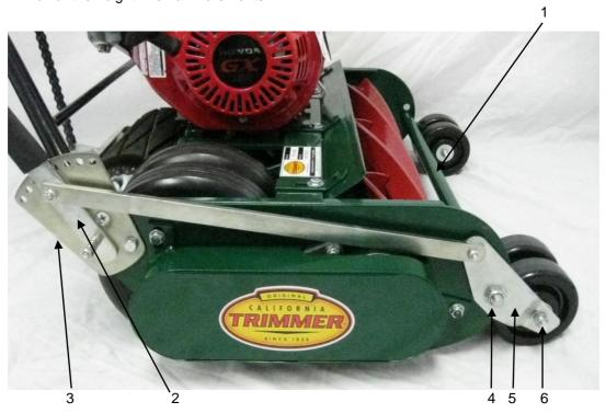
To change the range setting, take the "height adjustment lever" (no. 2) out of the holes of the "quadrant" (no. 3) and move it in the direction of the change. Back if the "caster bracket" (no.1) is being moved to the top hole or forward if the "caster bracket" (no.1) is being moved to the bottom hole. Loosen the "caster wheel nut" (no. 6).
