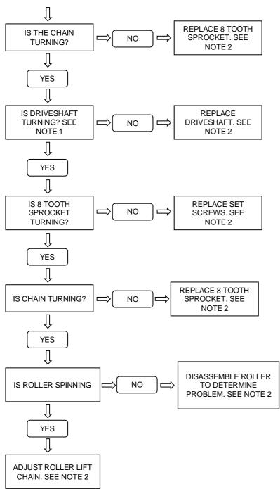
NOTE 1: LOOK AT SHAFT INSIDE 17 TOOTH OUSIDE SPROCKET. NOTE 2: SHUT OFF ENGINE BEFORE ADJUSTING.
