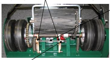
The clutch adjusting bolt has two nuts set together that hold the clutch forks and spring in position once it has been adjusted to the proper tension. The inner nut is for adjusting the tension of the spring and the outer jam nut, when tightened against the inner nut, secures the desired tension of the spring.
