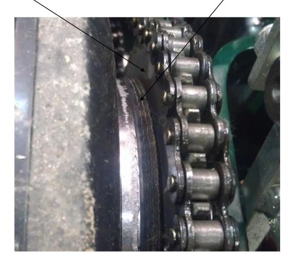
**Step 3** When proper clearance has been achieved retighten outer jam nut.
