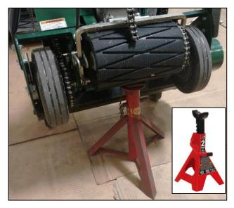
While blocking the front wheels, use the handles to lift/tip the unit forward and slide the jack stand under the drive roller sufficiently, then lower the unit down on to it (the roller will move upward and press against the frame). CAUTION: FUEL MAY LEAK IF TIPPED TOO FAR WHEN THE TANK IS COMPLETELY FULL.
