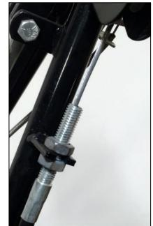
nut (lower) may be needed to provide adequate reach to connect the end to the lever. See pages 5-6 for final adjustment.
