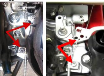
Step 11 – Install (New) Clutch Cable – Handle Side
