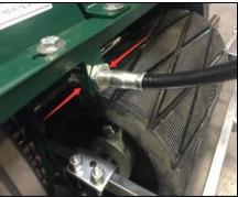
**STEP 9 – Install (New) Clutch Cable – Frame Side** It's best to immediately install the new cable at this time, so insert the new cable into the frame in the same position (equal threads on both sides), then place the cable end in position and insert the bolt (with the spring still connected) through the cable end and idler arm then install the nut.
