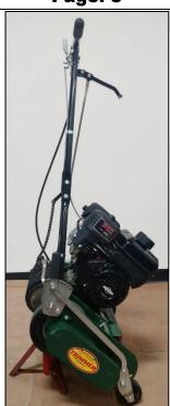
With the unit tipped forward and secured in place, access the connection bolt & nut and use 2 x 1/2" wrenches to loosen. **NOTE: The return spring is also held in place on then bolt head side of this connection.**
