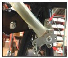
B. Remove air filter cover to access mounting clamp, loosen the screw to remove outer casing, then remove inner wire from throttle arm. NOTE: The end is "Z" shaped.
