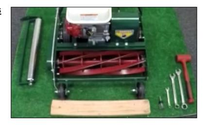
Begin by placing the board underneath the front part of the frame to elevate it and making sure it's evenly spaced / extending outward on each side. Next, move the height adjustment lever forward to the first position, which will expose the bracket / arm screw that needs to be removed.
