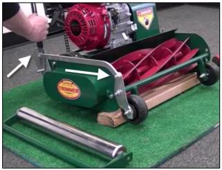
Using the 3/4" and/or adjustable wrenches, remove the axle nut, then use the 7/16" wrench and the Phillips head screwdriver to remove the nut and screw holding the height adjustment arm to the bracket.
