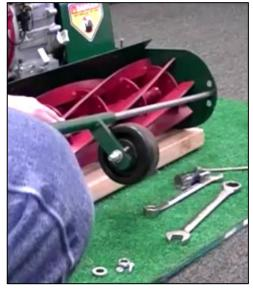
If needed, this is an opportunity to change the cutting height adjustment range by moving the axle to an alternate frame hole. On the current version of the RL20H series, the top set of holes are not used since the middle and lower holes provide the lowest and highest cutting heights. Move the axle to the lowest holes for a higher range or the middle holes for a lower range. Refer to the operating manual for details.
