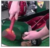
The bracket and the washers will slide off, then move the wheel housing out from the frame so it can be pulled off the axle bolt – which can stay in the frame.
