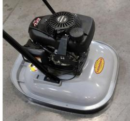
With the skirt in place, install the clamp brackets with 2 on the front, and 2 or 3 on the left and right side. NOTE: The deck and skirt may need to be pushed into place to fully seat together.
