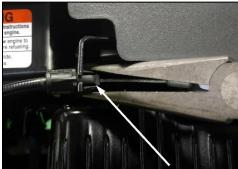
**STEP 5** - Install the kit's (longer) cable end by inserting the end onto the engine brake lever, then inserting the outer cable into the bracket. Install the additional handle section, secure with knobs, then re-install the engine stop cable adjuster and lever.
