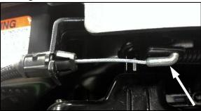
**STEP 4** - Remove the outer cable from the bracket – by using pliers to compress the locking tabs while pulling.
