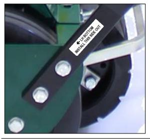
On the RH side, <u>use the new fasteners supplied</u> and place the spacer between the extension bracket and adjustment bracket (as shown in the image) to provide extra space for handle movement and position locking. Tighten all fasteners securely on both sides.
