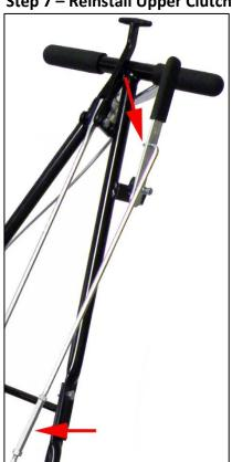
Add the longer connection nut to the upper rod, thread it back onto to the lower rod, and tighten until it can be inserted into the lever.
