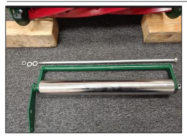
The new update is supplied as replacement roller sections and insert spacers that can be installed on the same axle / frame assembly as the original smooth version. The most effective way to approach the conversion is to remove the front roller frame from the mower and it's best to place wood blocks or a 2x4 under the front of the mower frame to raise it up for easier access. Start by disconnecting the height adjustment arm from the bracket, then remove the long
