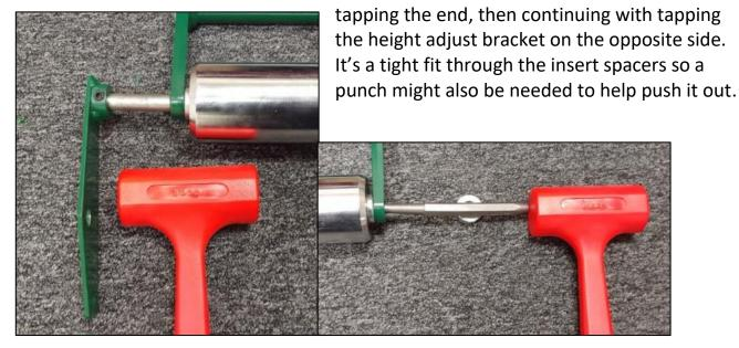
Once the shaft is out completely, it's recommended to clean and smooth the entire length (using sandpaper or steel wool). Place the new grooved roller sections together into the frame and begin inserting the shaft... again keeping in mind that it's a fairly tight fit through the insert spacers and will take some finesse (slight movement and perhaps some light tapping) to get it all the way through.
