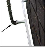
**#1. SIDE-TO-SIDE PIN...** inserts through the end / open chain roller. This is used for shortened chains and provides smaller increment lift adjustments.
