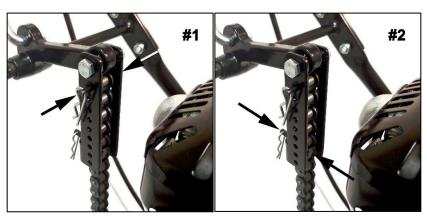
The drive roller's frame has 2 x heavy-duty springs pulling it downward to help maintain its traction on the ground, so the optimum setup – when the cutting height adjustment is set – is to have just a couple links of slack (where the chain connects) when the roller is down. This will provide the highest lift off the ground for the roller while allowing some additional downward movement for low spots...
