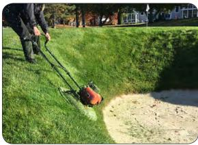
This lightweight yet powerful hover mower floats on a cushion of air and is designed to provide excellent cutting performance at steep angles for a wide variety of commercial, golf course and residential applications. It's extremely maneuverable as it can easily glide in multiple directions over grass surfaces and it mulches as it cuts so the fine clippings get to the soil surface.
