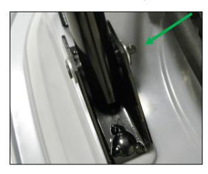
Attach the <u>upper handle</u> section to the lower handle section – with the stop lever facing forward – using the bolts and knobs as shown:
