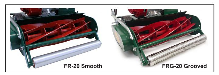
The front roller replace the standard caster wheels and provides a few advantages. First, this adds additional weight to the front of the mower for more stable tracking which is helpful for rougher yards. It also minimizes uneven cut from low spots and allows the mower to hang over the lawn edges and flower beds for extra close cuts. They are made of hard plated steel and have large sealed ball bearing for long life durability
