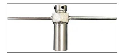
This tool is used for compressing the clutch spring when the installing it on to the drive shaft.
